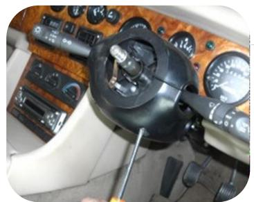
**Step 4.**Remove the cover from the lever unit.
